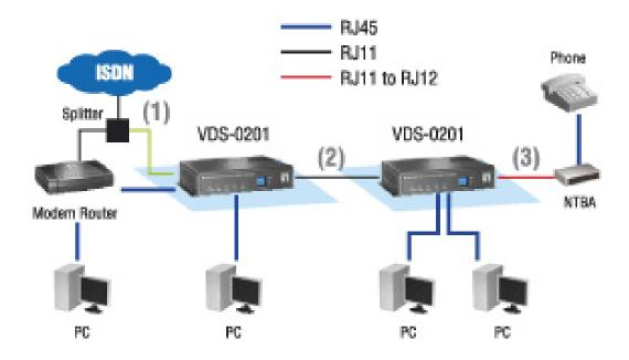
1) Cable for connection between ISDN Splitter and VDS-0201 Master:
