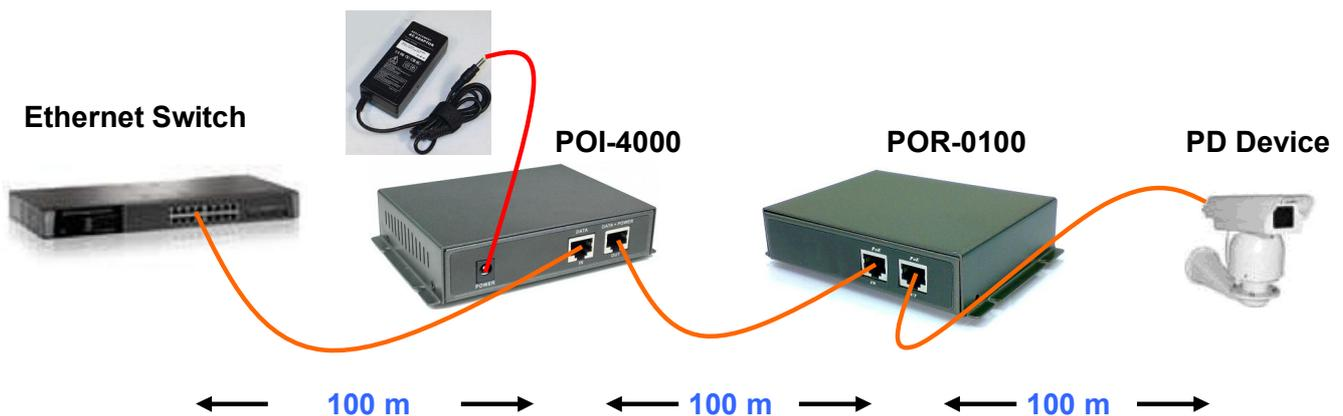
**\*\* Note:** If the Ethernet cable is not standard CAT5 cable, the POR-0100 may be working for shorter length than 100 meter.
