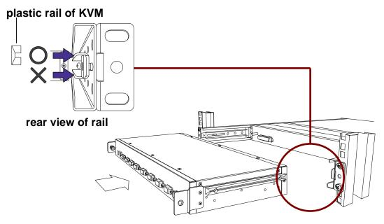
3. Tight thumb screw of bracket A up to fix KVM module in console and finish installation. (Both sides)
