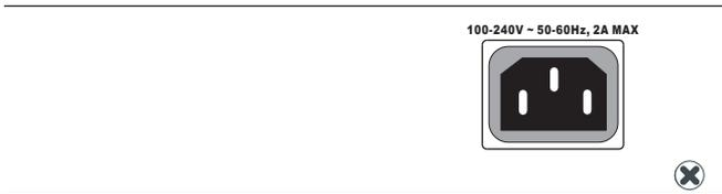
2. Plug the other end of the cable into a grounded, 3-pin, AC power source.
