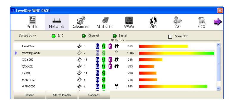
Sort by: Indicate that the AP list is sorted by SSID, Channel or Signal.
