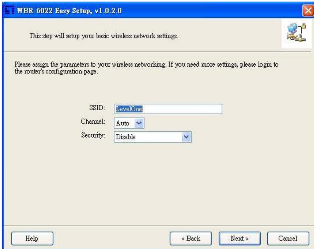
For wireless setting, the default SSID of wireless interface is “LevelOne”, default channel is 11, and default encryption option is “NONE”.
