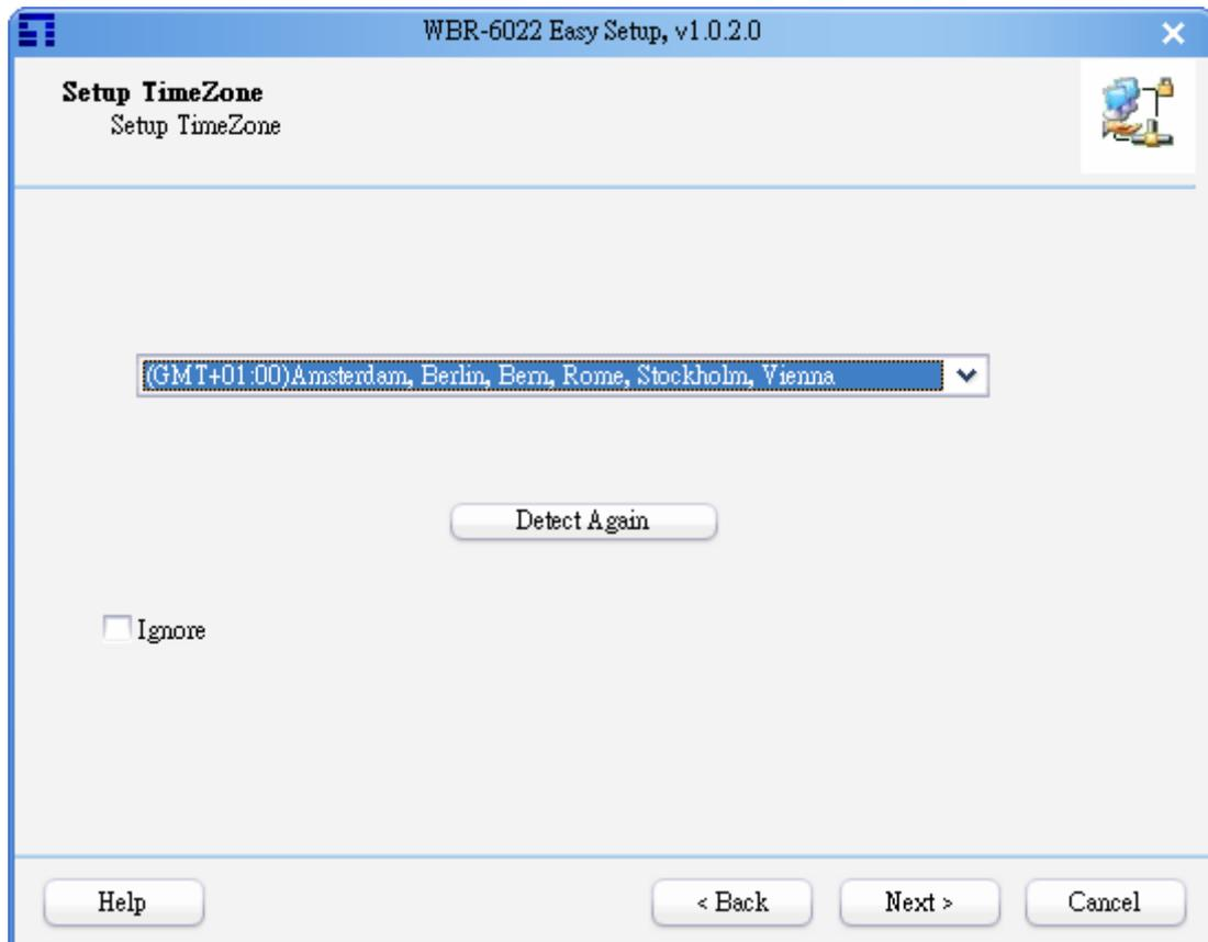
Then, you have to adjust the time zone. This router could manage the power by time scheduling, so we have to correct its system time.
