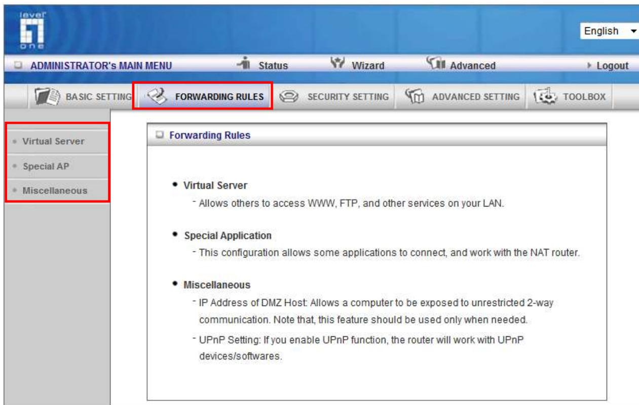
The port forwarding feature is required because the Wireless Router's NAT (Network Address Translation) will block incoming traffic from the Internet to the LAN if the specific port mapping is not set up in the NAT table.
