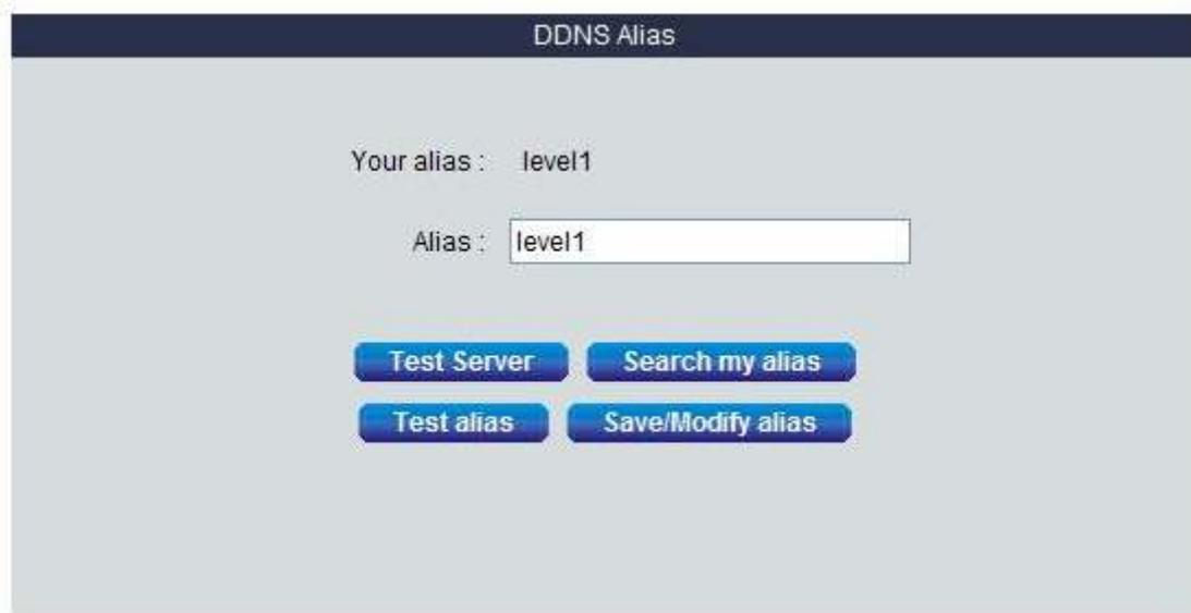
**DDNS Alias:** Key in your preferred alias name and press “Test alias” button to check it is valid or not. Press the “Save/Modify alias” button then the alias setting process is done. Then you can try to open the IE browser and input the full DDNS address. The format is “alias”+“level1dns.net”, here have some example for reference.
