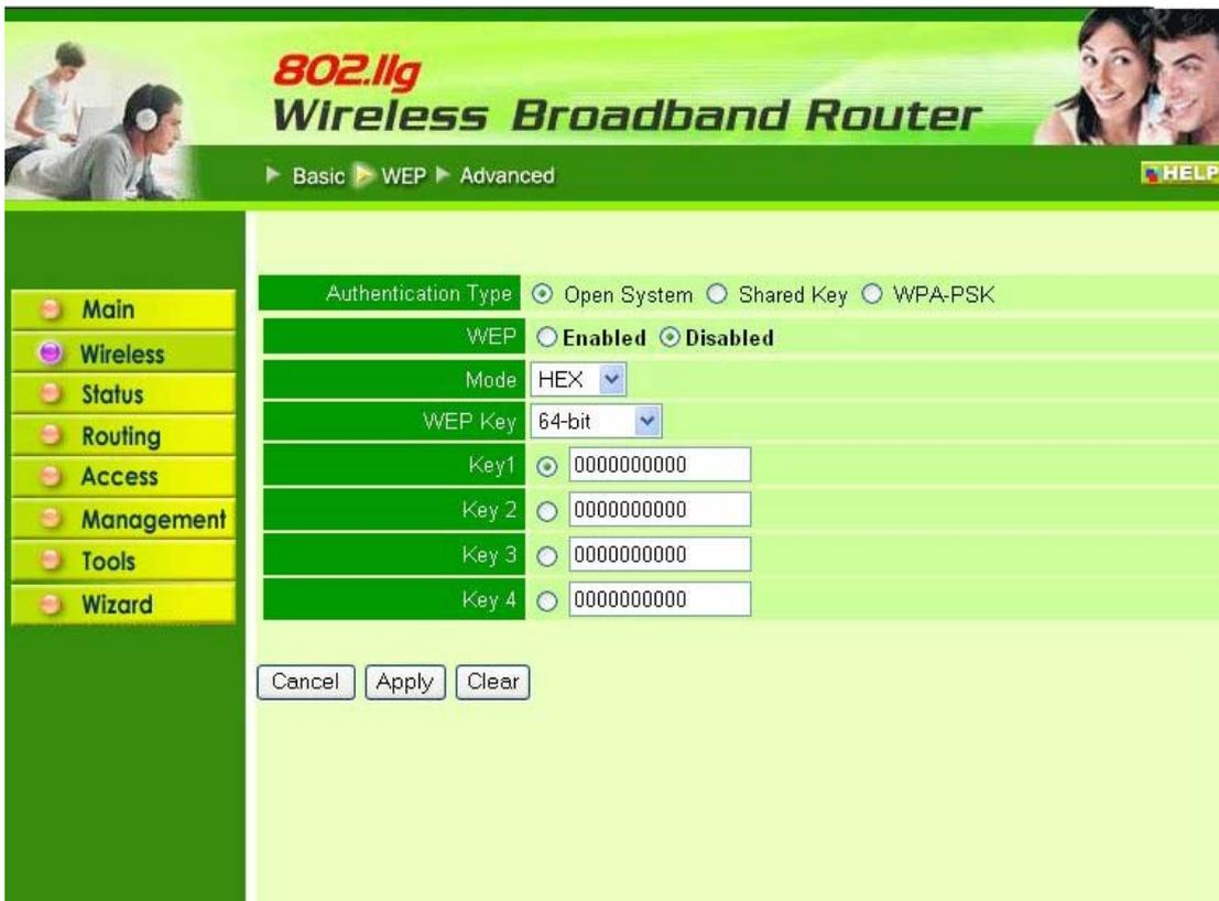
**Authentication Type:** The authentication type default is set to open system. There are three options: Open System; Shared Key and WPA-PSK..
