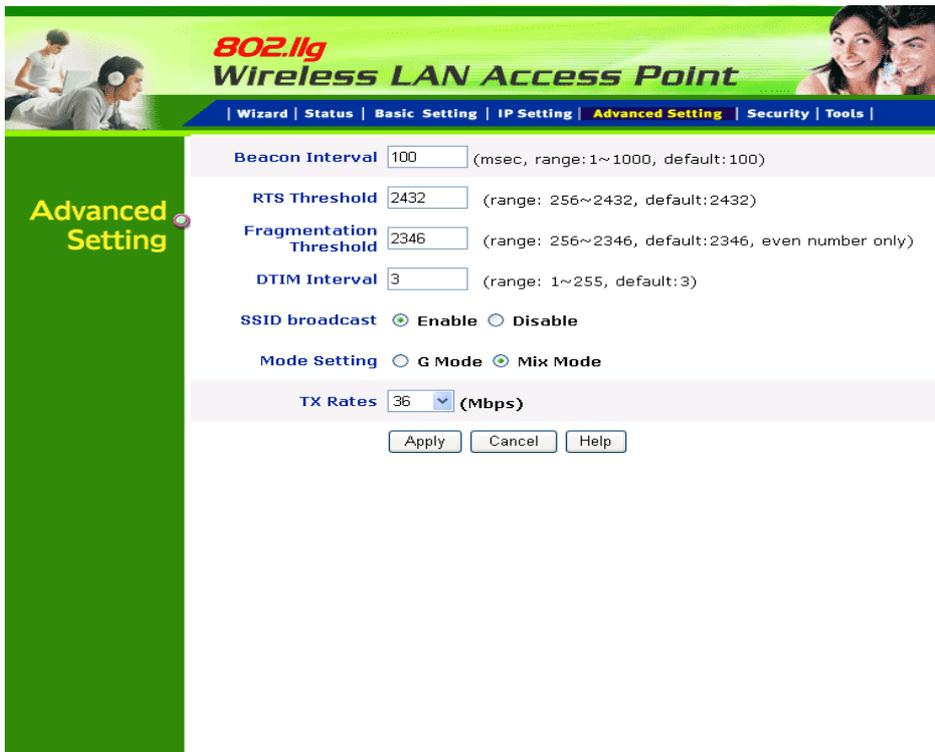
**Beacon Interval:** To set the period of time in milliseconds that AP sends out a beacon. Default is 100 milliseconds.
