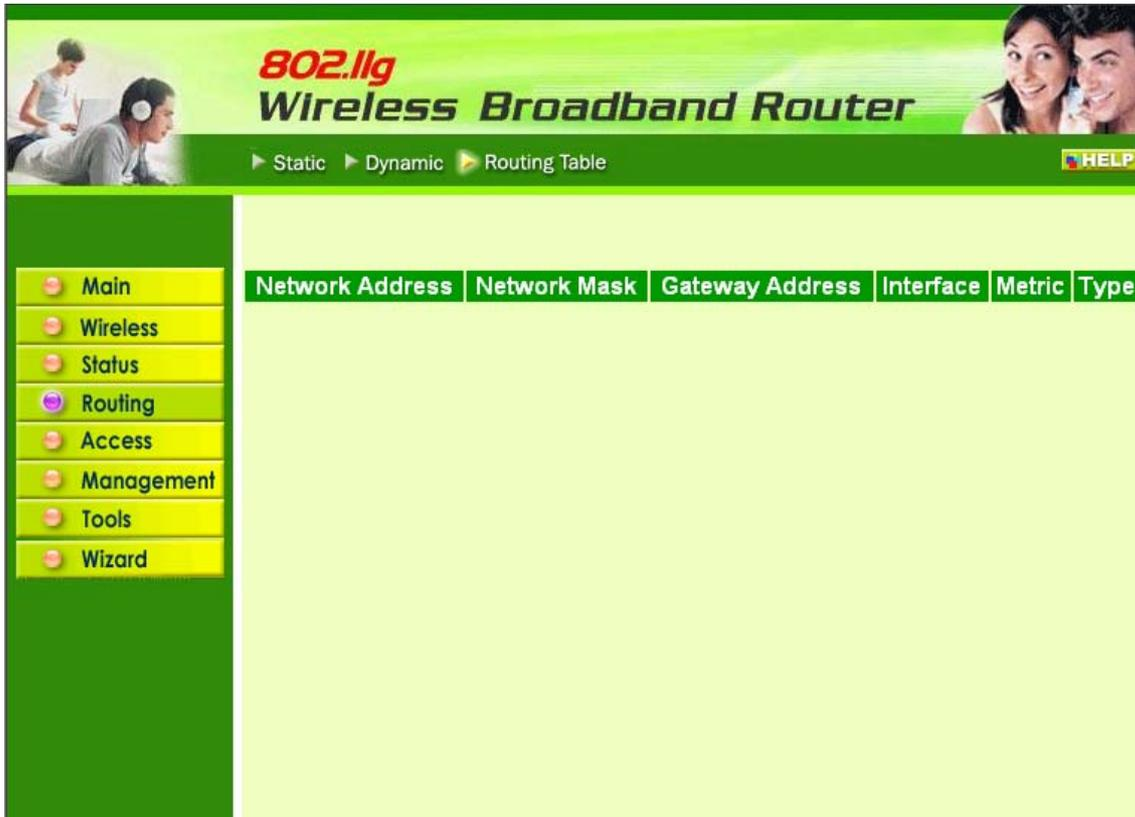
**Network Address:** Displays the network IP address of the connected node.
