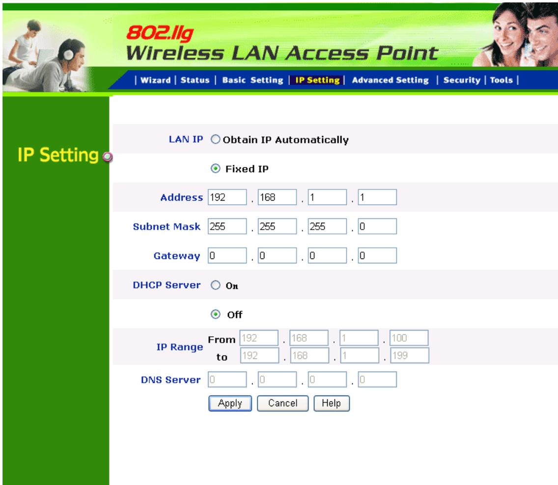
The screenshot shows the configuration interface for an 802.11g Wireless LAN Access Point. The page has a green header with the product name and a navigation menu. The main content area is titled "IP Setting" and contains several sections for configuration:
