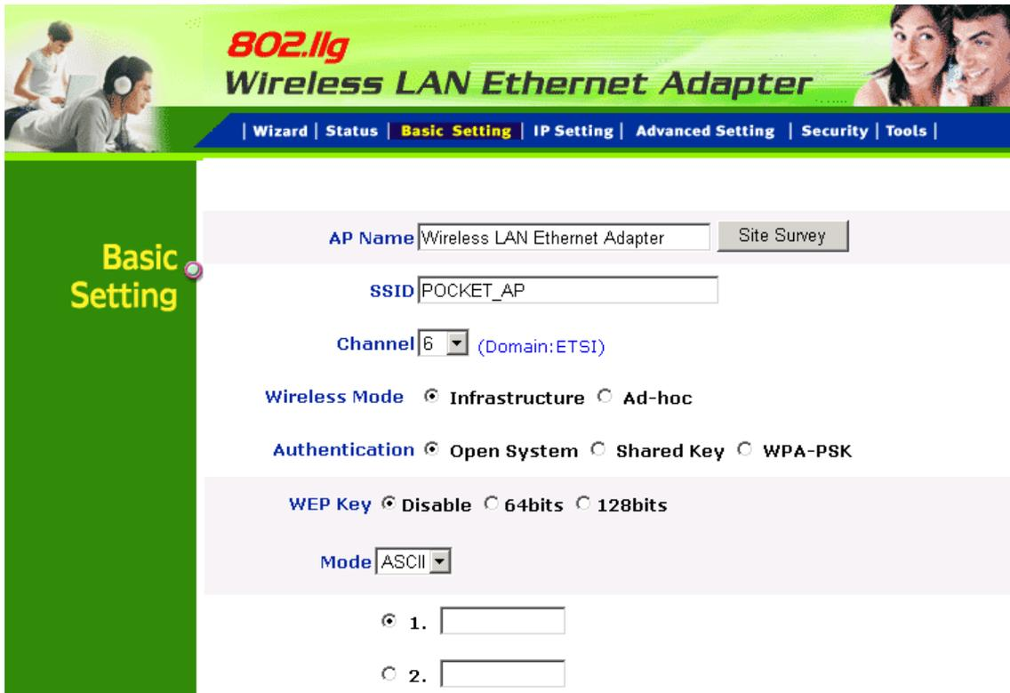
The screenshot shows the 'Basic Setting' page for the 802.11g Wireless LAN Ethernet Adapter. The page features a green header with the product name and a navigation menu. A green sidebar on the left contains the text 'Basic Setting'. The main content area is a light gray form with various settings:
