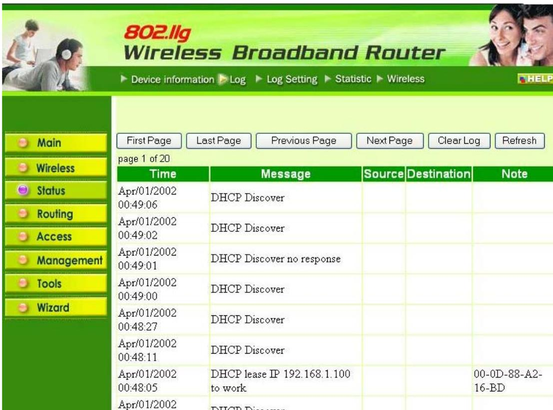
The screenshot shows the web interface of an 802.11g Wireless Broadband Router. The top navigation bar includes links for Device information, Log, Log Setting, Statistic, and Wireless. A sidebar menu on the left contains options: Main, Wireless, Status, Routing, Access, Management, Tools, and Wizard. The main content area displays a log table with the following data:
