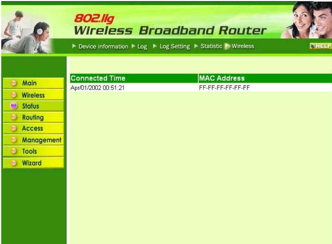
**Connected Time:** How long the wireless device has been connected to the LAN via the router?
