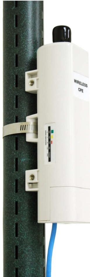
**Figure 10 Pole Mounting – Step 3**
