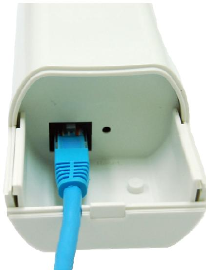
**Figure 4 Cable Connection**
