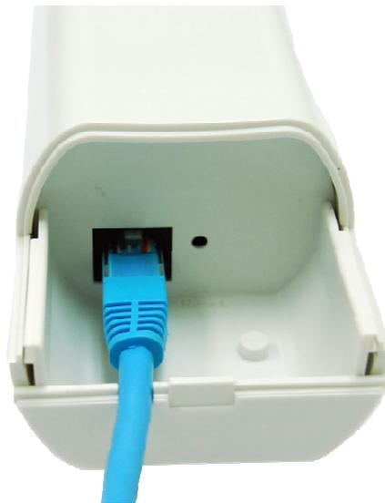
**Figure 4 Cable Connection**
