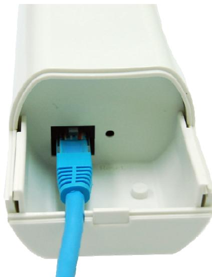
**Figure 4 Cable Connection**
