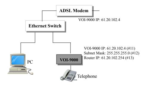
If you forgot the current VOI-9000 address, you may enter the new IP address from telephone by using #11 commands.
