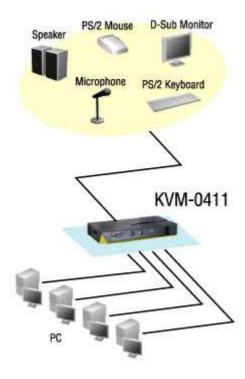
4. Power up the connected computers one by one. After your computers are powered up, the keyboard and mouse will be recognized and now you can begin operating the KVM switch.
