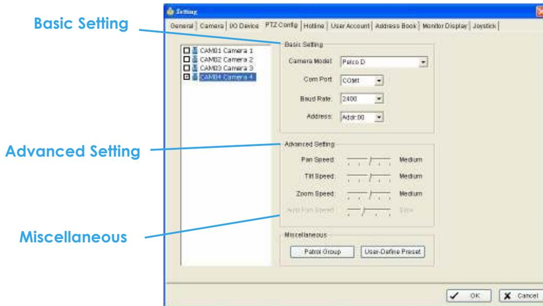
Install PTZ cameras and follow the instruction of the camera manufacturers. A PTZ camera is usually connected to the PC with RS-485/RS-422.
