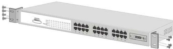
Figure 2-4. Attach mounting brackets with screws
