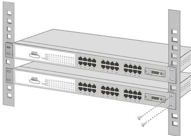
Figure 2-5. Mount the switch in an EIA standard 19-inch Rack
