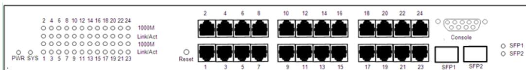
Figure 1-1 Front Panel of GEL-2460
