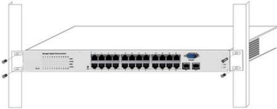
Figure 2-1 Installing the Switch in a Rack
