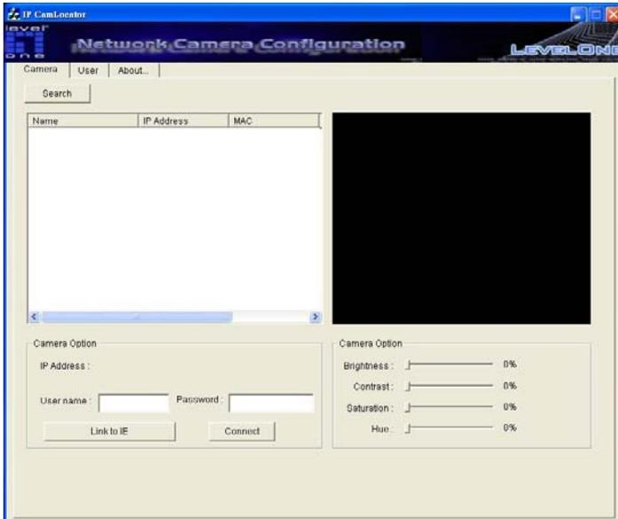
The IP addresses shown in the "IP Address" field reflect those on the local network. They may be from the DHCP server. If there is no DHCP server, the camera will try to find a free IP address (this takes from 15 second to 3 minutes, depending on the LAN status). The method of finding IP address is seeking from 192.168.0.2, to 192.168.0.254. If any of the address inside this range is free, the Network Camera will be assigned to this IP address, and its subnet mask would be 255.255.255.0.
