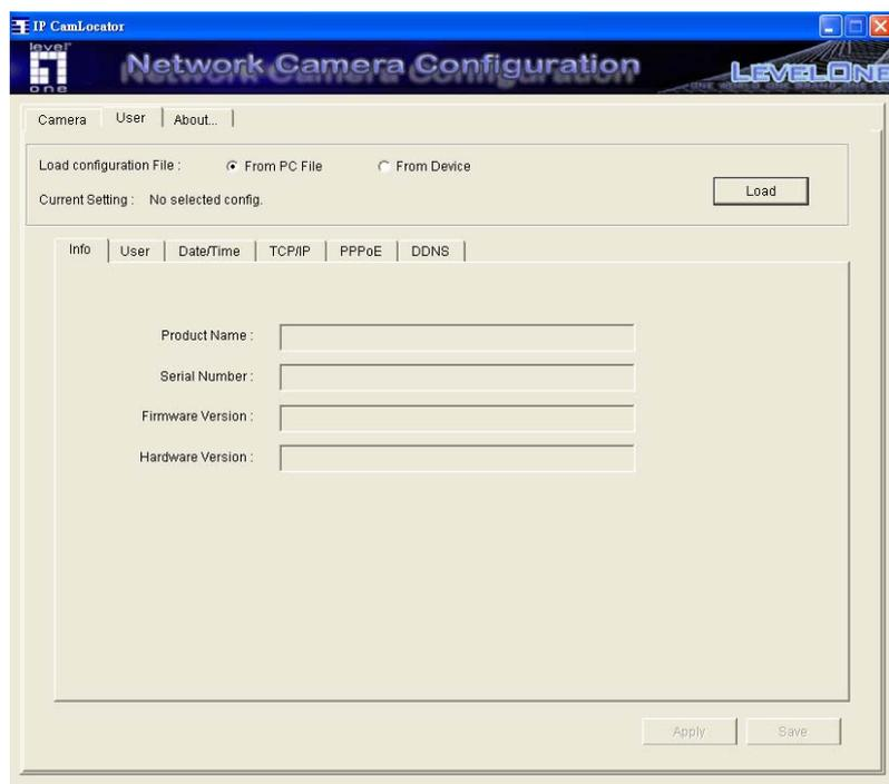
**Load configuration File** : Select **From PC File** or **From Device**, the former one can load information of downloaded configuration file and the latter one can load Network Camera configurations in the network.
