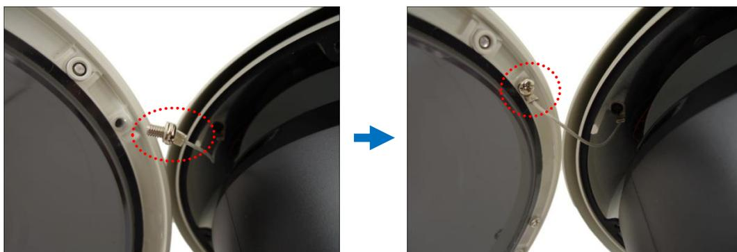
5. Tighten the four (4) screws to close the dome cover.
