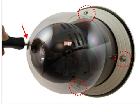
2. Carefully lift the cover. Using a screwdriver, remove the screw to detach the cover from the camera.
