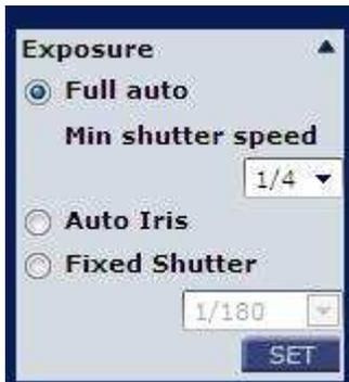
The exposure is the amount of light received by the image sensor and is determined by the width of lens diaphragm opening, the amount of exposure by the sensor (shutter speed) and other exposure parameters. With this item, users can define how the Auto Exposure function works.
