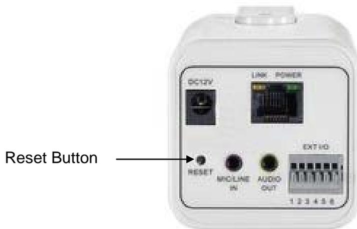
The Reset Button can be used to reboot the camera or restore it to factory default settings. If the camera experiences a problem, rebooting the camera may correct the problem. If the problem remains, please restore the camera to factory default settings and reinstall the software.
