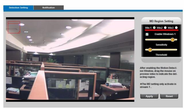
**Detection Setting:** Select and enable the motion detection windows function. Easier to trigger event by higher the sensitivity value and lower the Threshold value.
