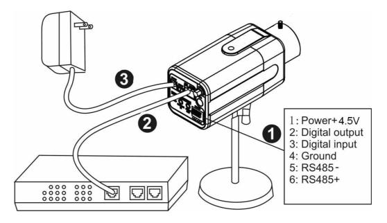
Please check your product package contains all the accessories listed in the foregoing Package Contents. Depending on the user's application, an Ethernet cable may be needed. The Ethernet cable should meet the specs of UTP Category 5 and not exceed 100 meters in length.
