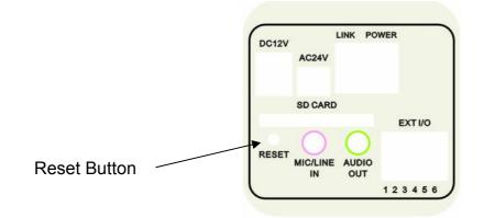
The reset button is used to reset the system or restore the factory default settings. Sometimes resetting the system can return the camera to normal operation. If the problems remain after reset, please restore the factory settings and install it again.
