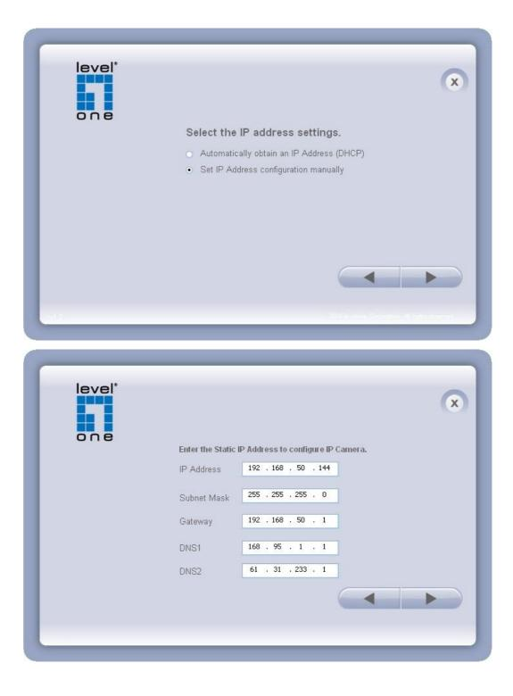
5. After finish setting, the connection successful or fail showed. If connection failed, user can either try again or quit the installation. User can either select "Start Web GUI" to continue or click "X" on the top right of the screen to finish the installation.
