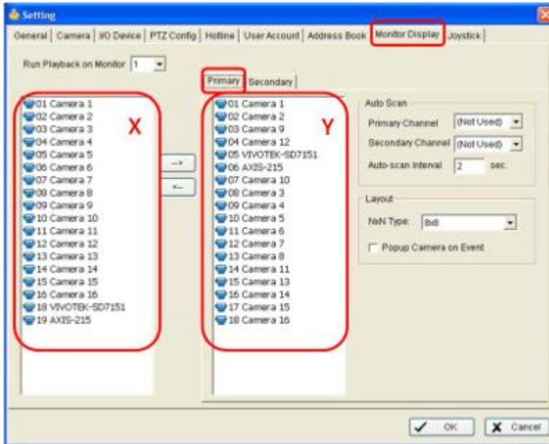
7.) Click on [Secondary] and pick the cameras to be displayed on the secondary monitor
