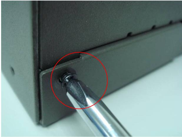
7. Unscrew the module slot cover at the back.
