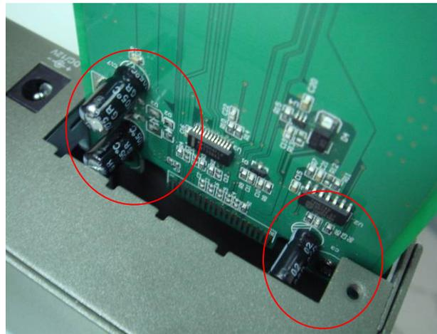
11. Be careful not to bend or damage capacitors while inserting.
