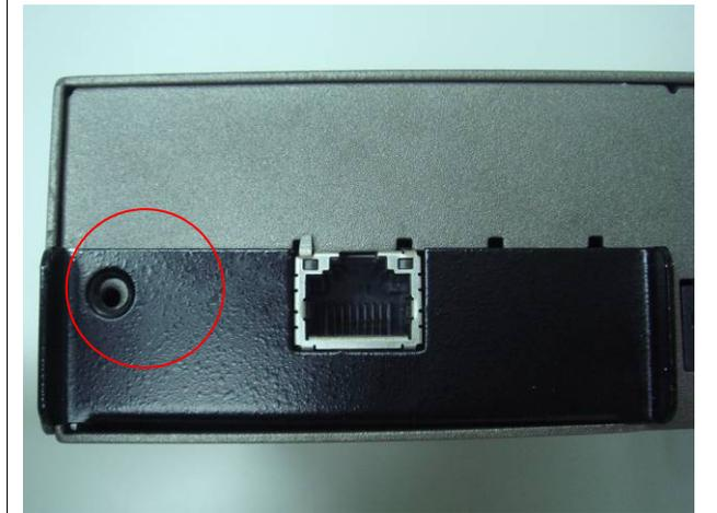
12. When correctly inserted, there is a screw hole at the upper left hand corner.
