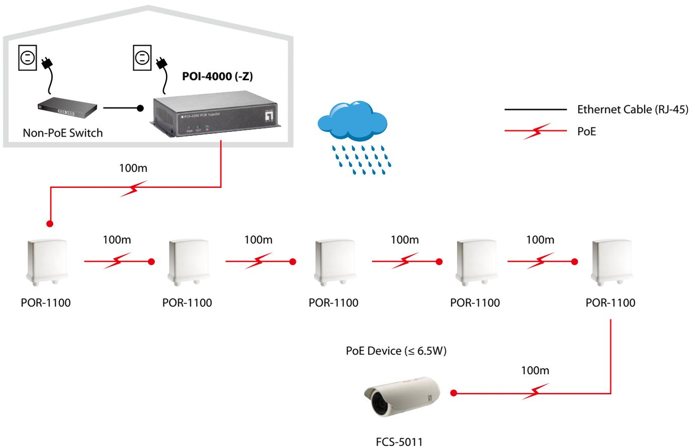
Note: These distances are typical results when used with 18~19Ω 24 AWG Cat.5 Cable
